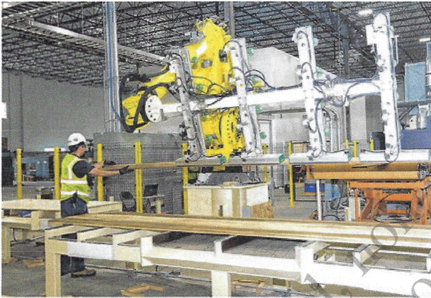
CHARLOTTE KESL FOR WSJ (3) An industrial robot that feeds boards into an assembly line is tested at InventWood's Frederick, Md., facility.
